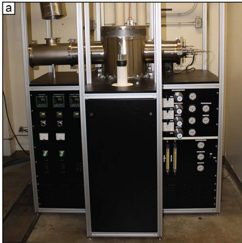
UC Irvine Low Velocity Burner Rig (Currently optimized for Hot Corrosion Studies)
